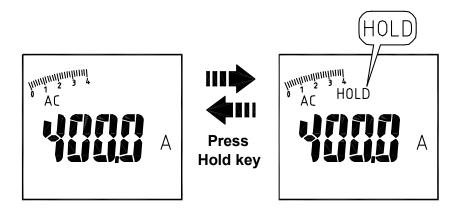
**SMART HOLD**: The meter will beep continuously and the display will flash if the measured signal is larger than the reading held on the display. (for V, A, W, and Flex AC current function).
