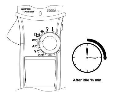
The meter can work again by turning it on from the OFF position.
