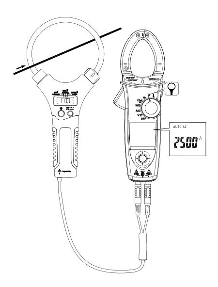
Note - Measure a known current to make sure that the ICA10T / ICA18T Flexi Current Probe and IPM 240F operate correctly.
