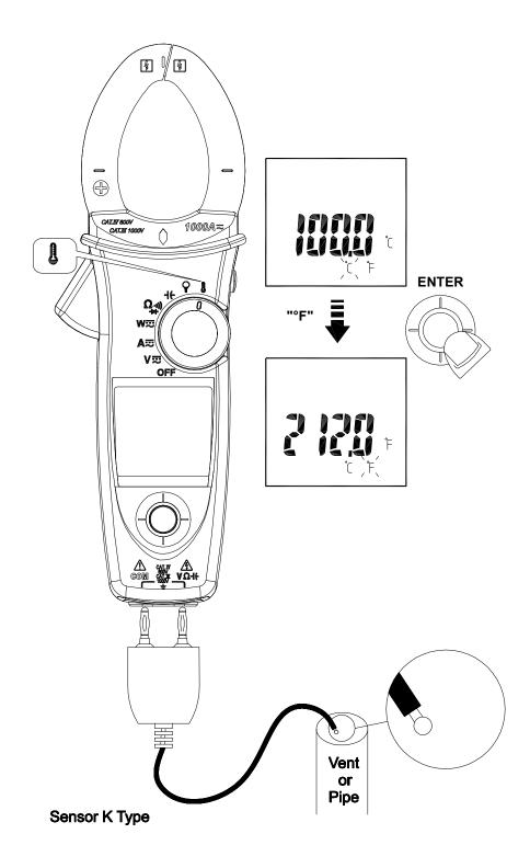
Do not take any high voltage measurement prior to accurate °C/°F measurements.
