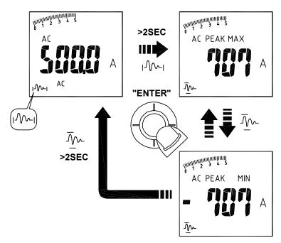
In PEAK HOLD mode, the meter is activated to save the positive peak value and the negative peak value. Positive peak value is displayed in PEAK MAX mode. Negative peak value is displayed in PEAK MIN mode.
