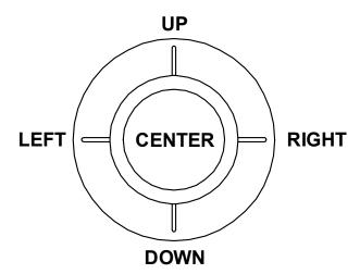
The Navigator key has 5 directions of switch on the display, toggle the navigator key to select the desired feature and to activate the feature by a simple click.
