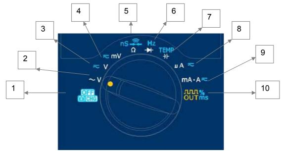
Figure- 3 Rotary Switch for selecting function
