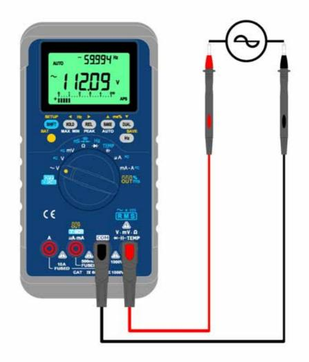
Figure- 42 Line power Voltage measurement
