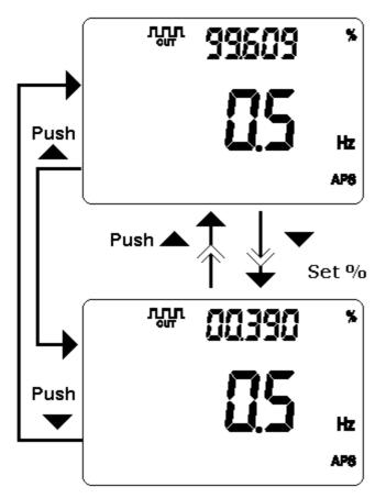
Figure- 24 Duty Cycle adjustment for Square Wave
