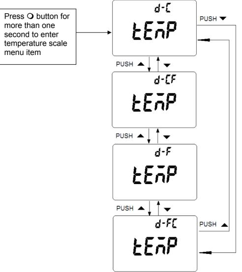
Figure- 14 Temperature Unit Setup
