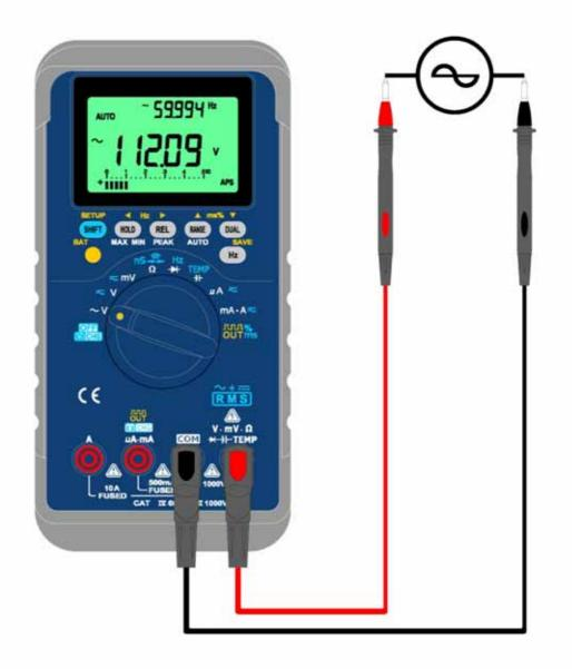
Figure- 1 Dual display for ACV/ Hz Measurement
