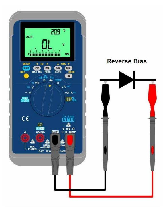
Figure- 53 Reverse Bias of Diode Measurement
