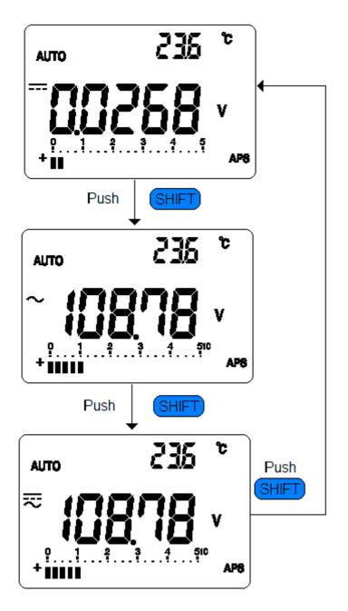
Figure- 40 Shift V function by Blue button
