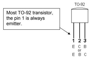
Figure- 55 TO-92 Transistor
