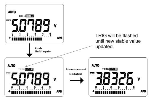
Figure- 31 Trigger Hold
