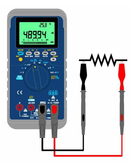
Figure- 51 Conductance measurement
