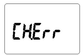
Figure- 27 Charge Terminal Alert
