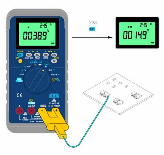
Figure- 60 Surface temperature measurement
