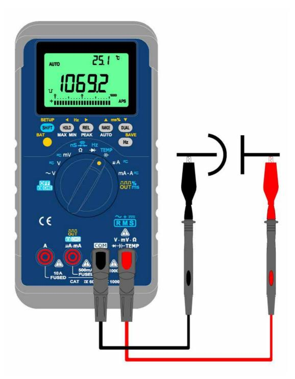
Figure- 54 Capacitance measurement
