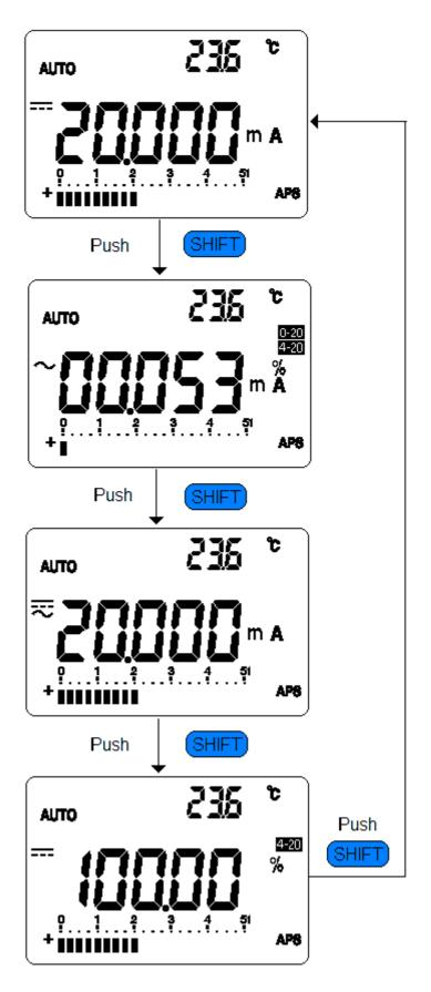
Figure- 41 Shift mA function by Blue button
