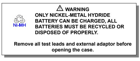
The meter is powered by 9 V battery, be sure to used specified battery. To ensure the specification specified, it is suggested to replace battery immediately as the sign of **G** low battery is displayed and flashing. If your meter has specified rechargeable battery inside, please go to how to charge battery. Following procedures for battery replacement:
