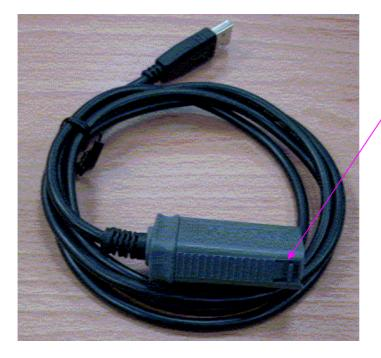
Always press second snap slightly to remove the cable from communication port of the meter.
