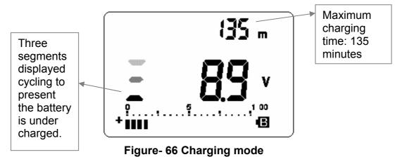
7. The charge end message (C-End) will be indicated on secondary display as the charging cycle has been finished. The trickle charging current still
