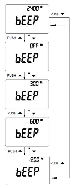
Figure- 13 Driving frequency of Beeper setup
