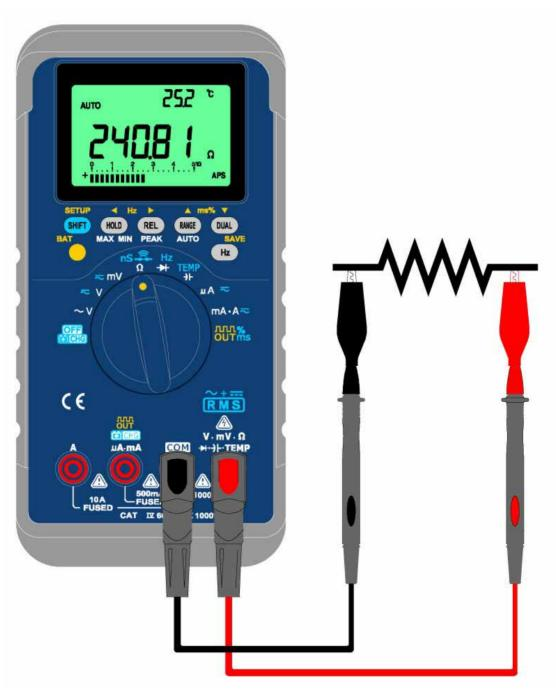
Figure- 50 Resistance measurement
