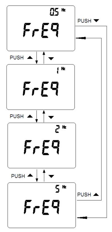
Figure- 12 Minimum Frequency Setup
