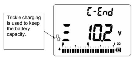
Figure- 67 Charge end and Trickle state
