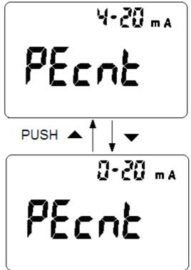
Figure- 11 The % scale Setup for mA measuring
