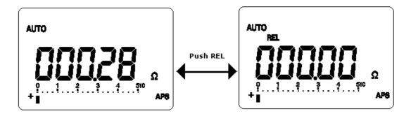
Figure- 33 Relative (Zero) Operation
