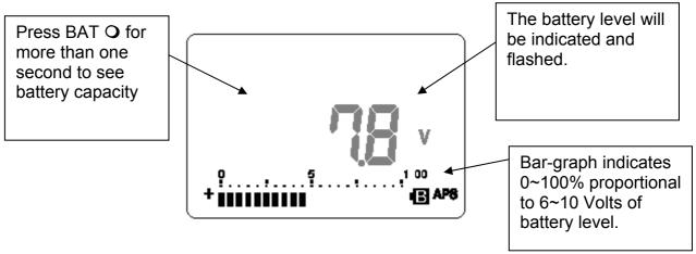
Figure- 28 Capacity check of battery
