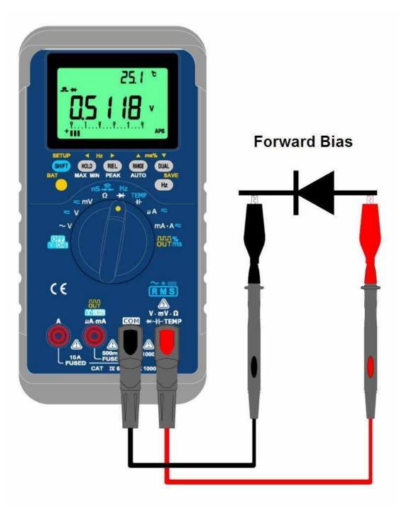
Figure- 52 Forward Bias of Diode Measurement
