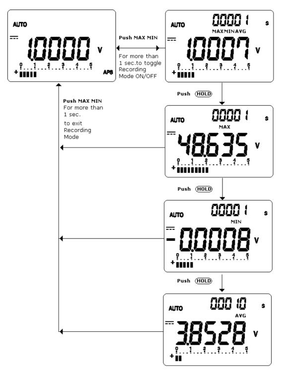
Figure- 29 Display of Dynamic Recording
