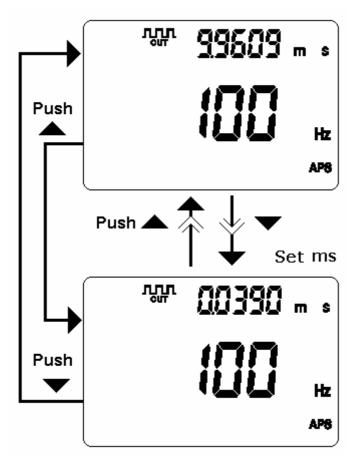
Figure- 25 Pulse width adjustment for Square Wave
