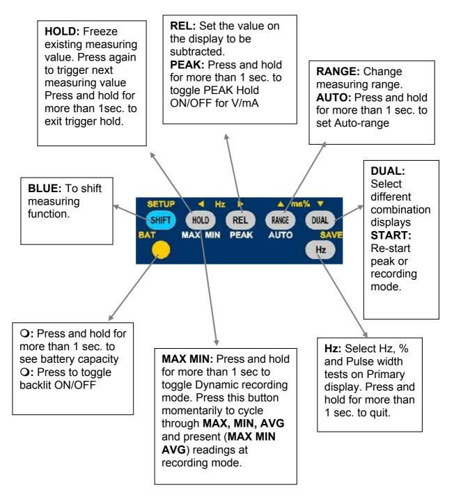
**Figure- 5 Pushbuttons**
