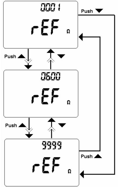
Figure- 21 Reference Impedance for dBm
