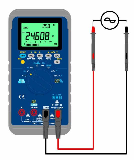
Figure- 43 Check the power source of transmitter
