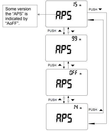
Figure- 17 Auto power saving setup
