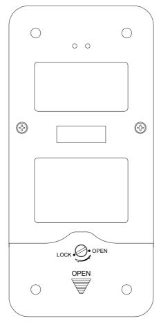
2. Turn the screw on the battery cover form LOCK to OPEN position by counterclockwise.
