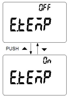
Figure- 16 Enable Environment Temperature display
