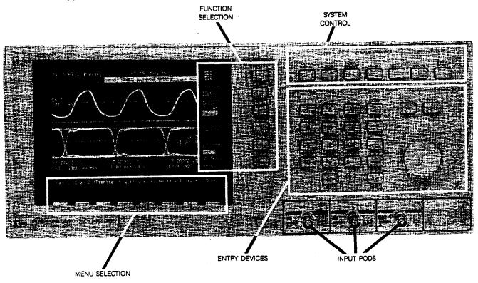
Figure 7-1. HP 54100A/D Front Panel
