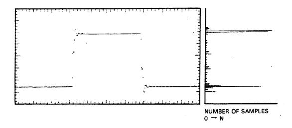
Figure 7-3. The Histogram of a Waveform.
