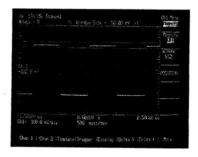
Figure 7-20. Magnify Window in the Normal Mode
