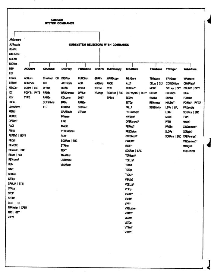
Figure 9-1. Programming Command Tree
