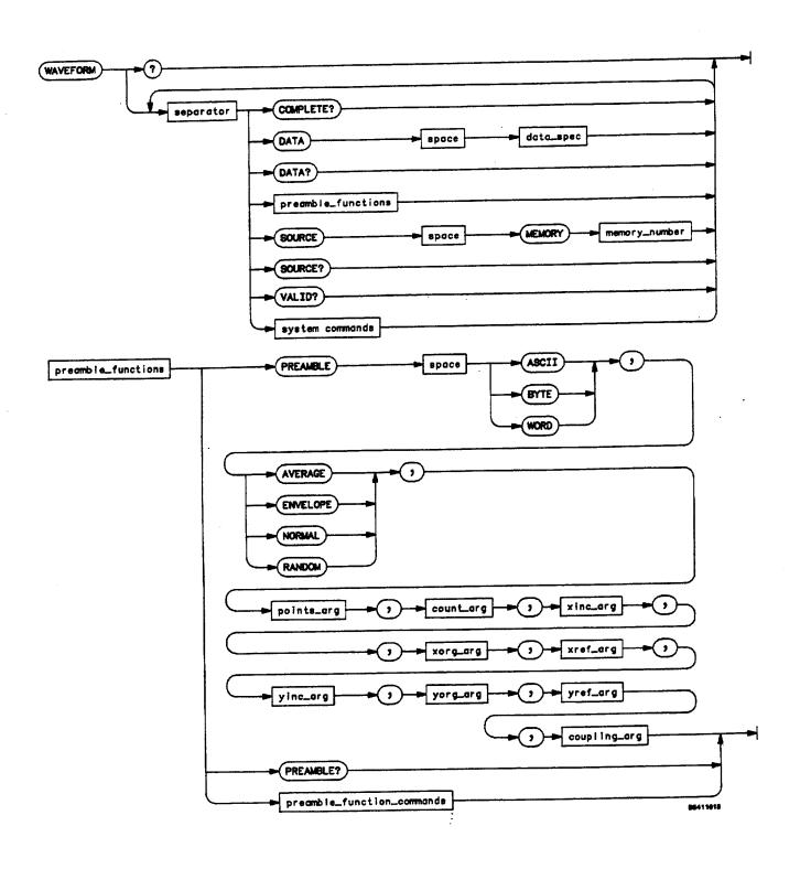
Figure 10-13. Waveform Subsystem Commands
