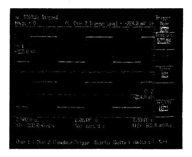
Figure 7-15. Split Screen with Trigger on Chan 2
