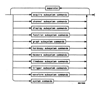
Figure 10-1. Command Set Syntax Diagram.
