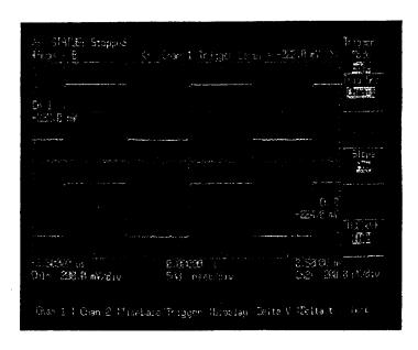
Figure 7-14. Split Screen with Trigger on Chan 1
