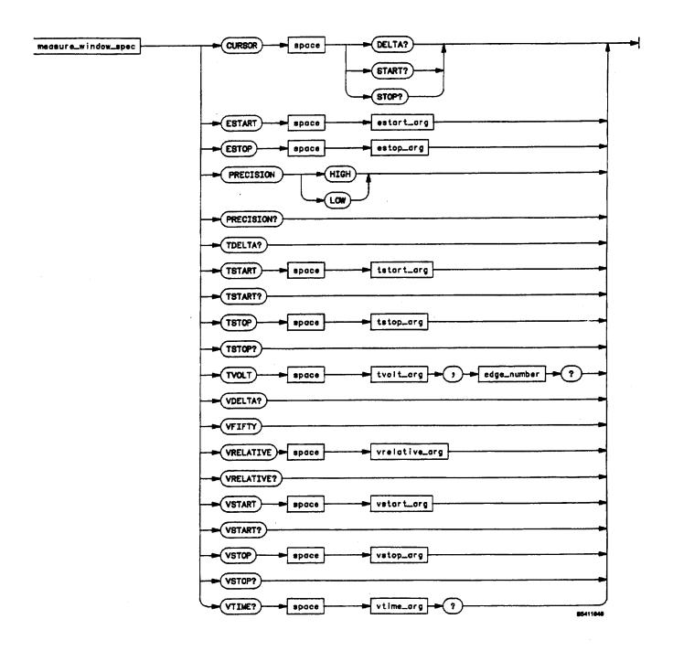
Figure 10-10. Measure Subsystem Commands
