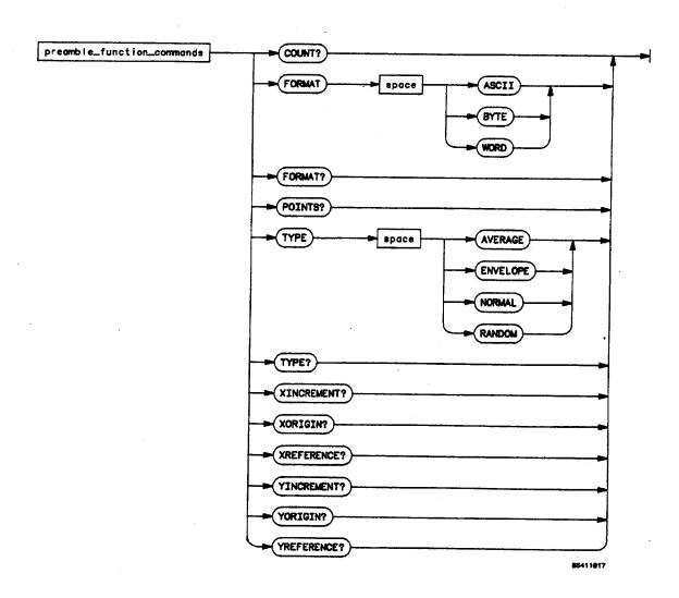
Figure 10-13. Waveform Subsystem Commands
