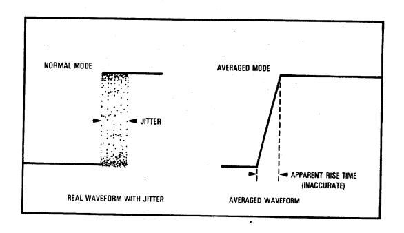
Figure 7-12. Time Jitter with Normal/Averaged Mode.
