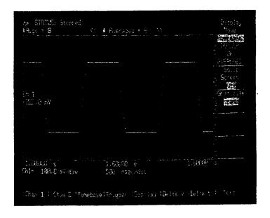
Figure 7-10. Time Jitter in the Averaged Mode
