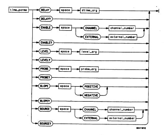
Figure 10-12 Trigger Subsystem Commands
