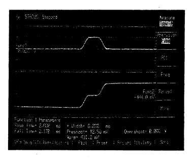
Figure 7-29. Automated Measurements on Func 1.
