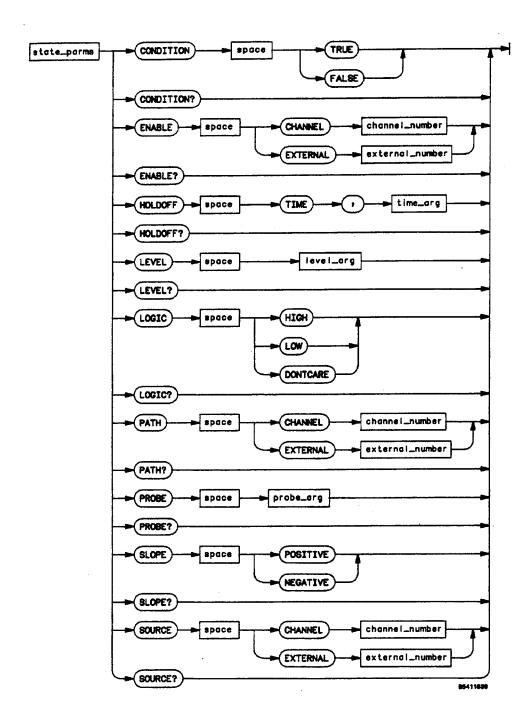
Figure 10-12 Trigger Subsystem Commands
