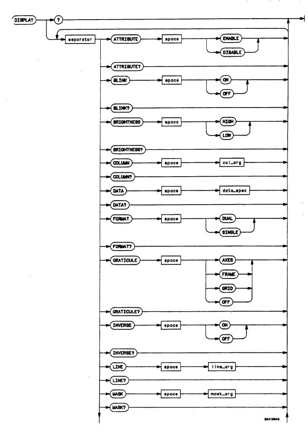
Figure 10-5. Display Subsystem Commands
