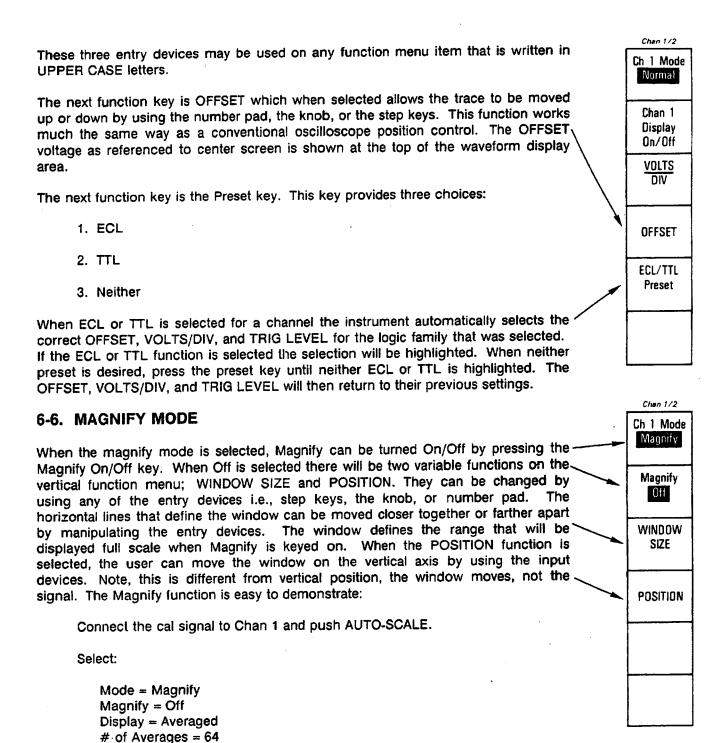
Alternately select and adjust the WINDOW SIZE and POSITION so the window is about the pulse top. When Magnify is turned On the portion of the signal that was defined by the window will fill the display. The vertical sensitivity or offset for the magnified display is shown at the top of the waveform display area.
