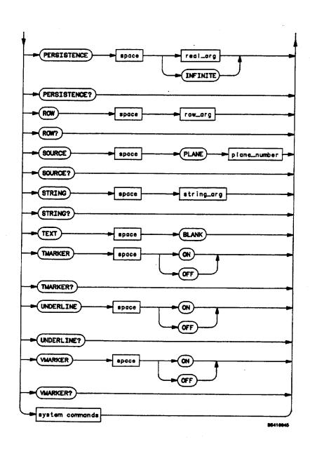
Figure 10-5. Display Subsystem Commands
