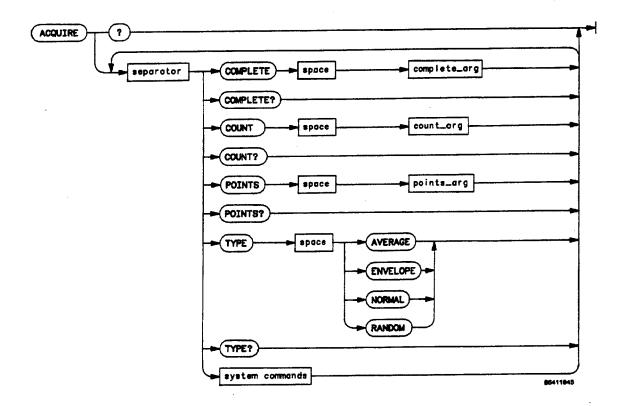
**COMPLETE\_ARG** := An integer from 0 to 100, specifying, in percent, the number of buckets that must be filled before acquisition is considered complete.
