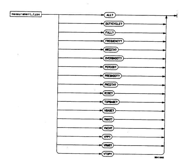
Figure 10-10. Measure Subsystem Commands
