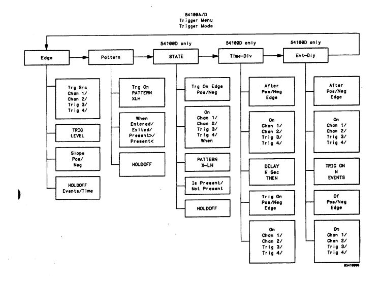
Figure 6-3. 54100A/D Trigger Menu
