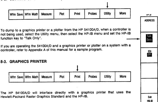
After the HP 54100A/D has been connected to the graphics printer and the configuration switch has been set to the LISTEN ALWAYS mode, select the Print menu on the HP 54100A/D.
