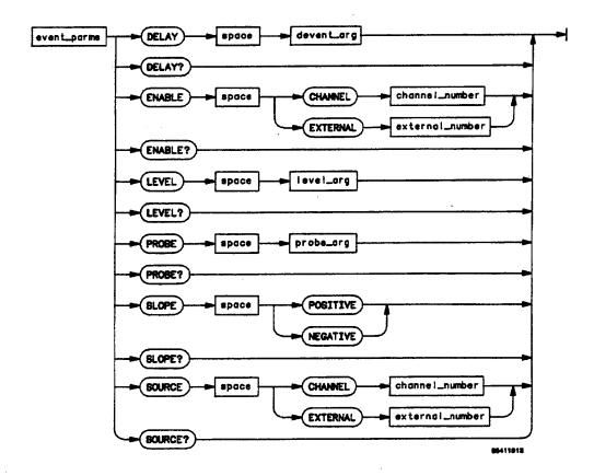
Figure 10-12 Trigger Subsystem Commands
