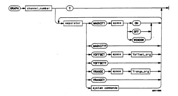
YOFFSET\_ARG = A real number less than or equal to the vertical range.
