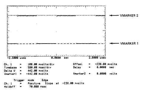
Figure 7-2. Manual Vmarker Measurement
