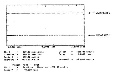
Figure 7-4. Auto Top-Base Voltage Measurement
