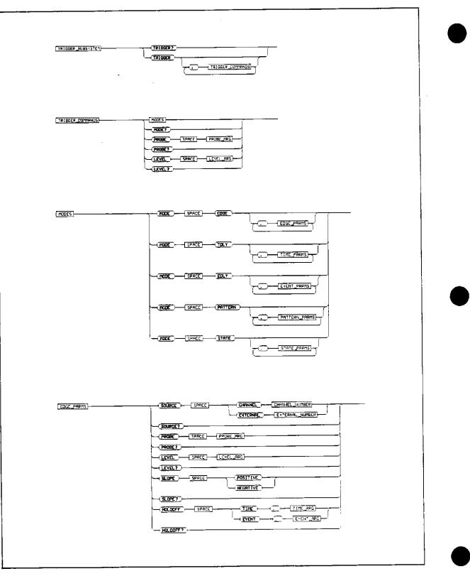
Figure 10-9(A). Trigger Subsystem Commands
