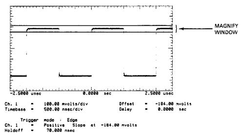
Figure 7-20. Magnify Window in the Normal Mode
