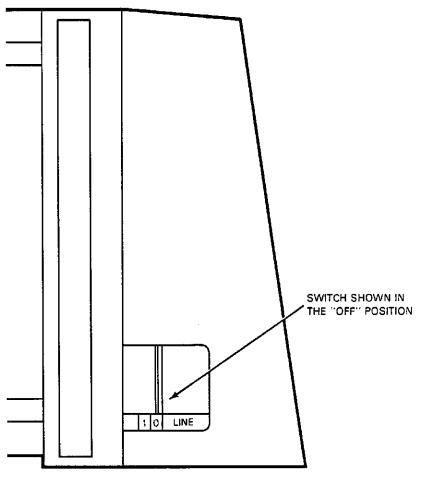
Figure 4-3. Front Panel Power Switch
