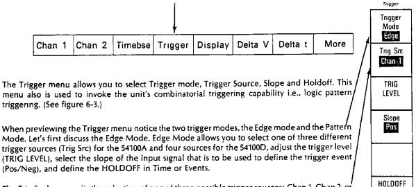
The Trig Src key permits the selection of one of three possible trigger sources; Chan 1, Chan 2, or the external trigger input (Trig 3). Note: the 54100D has a second external trigger input (Trig 4) for a total of four trigger sources.
