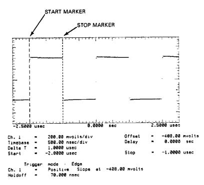
Figure 7-7. Manual Time Interval Measurement
