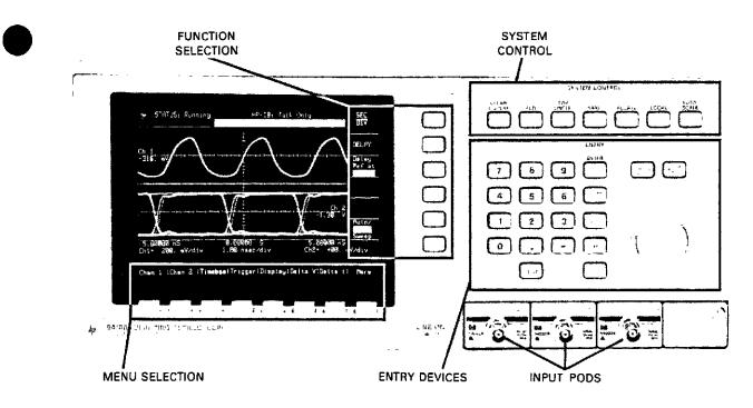
Figure 5-1. 54100A, D Front Panel
