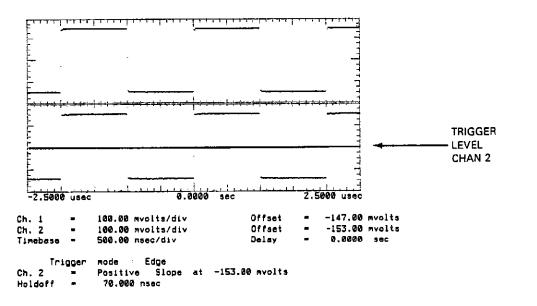
Figure 7-15. Split Screen With Trigger On Chan 2
