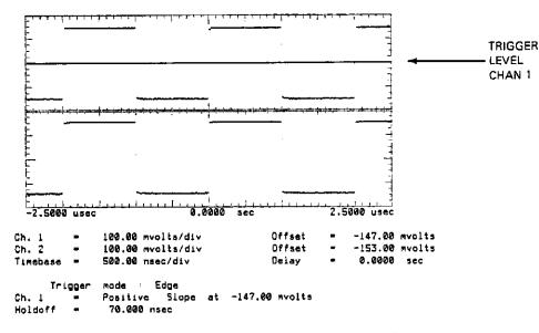
Figure 7-14. Split Screen With Trigger On Chan 1
