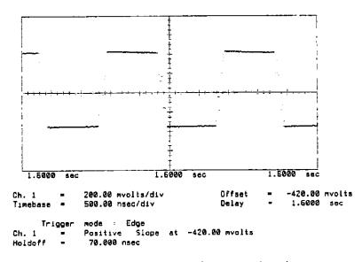
Figure 7-10. Time Jitter in the Averaged Mode
