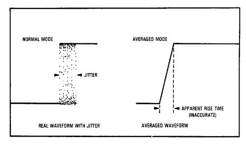
Figure 7-12 Time Jitter With Normal/Averaged Mode
