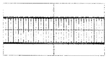
Figure 7-13. Auto Sweep Mode With Delay > 50 ms
