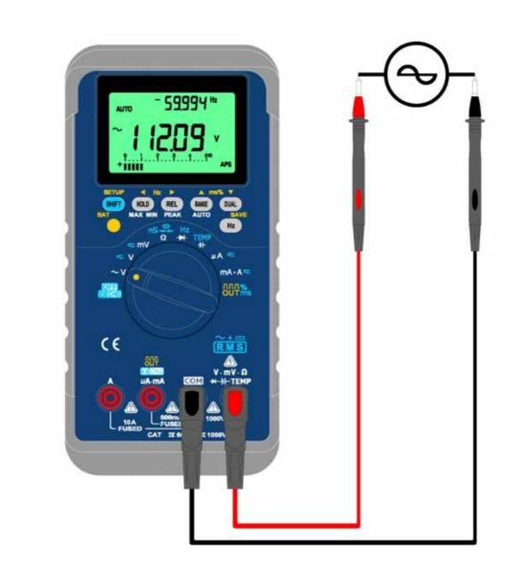
Figure- 1 Dual display for ACV/ Hz Measurement
